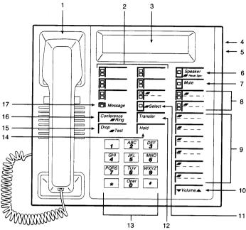
Figure 1. 7406 Plus Voice Terminal (With Display)
